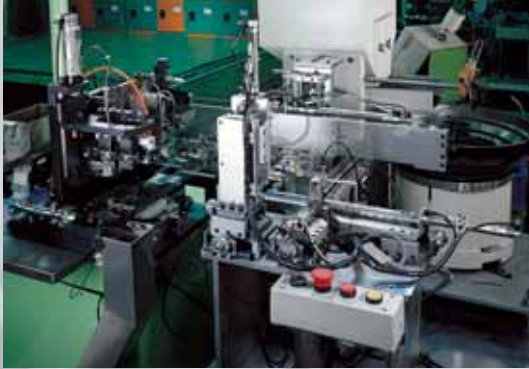
整修入彈簧機 自行開發設備,可縮短流程,減少暫存。 Trimming & Spring Loading Machine. Designed and developed by NAK to shorten manufacturing process and register. 修正型投入機 自社開發の設備。工程の短縮が可能で一時在庫が減少。
